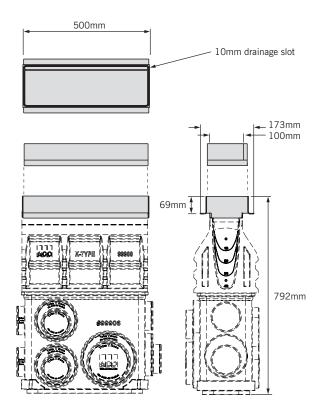
Note: Access units to allow access for maintenance to be located at both ends of the drain, at the outlet and/or spaced at 20-30 metre intervals.
